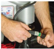
Wiring is reduced to a minimum and installs easily using a one plug connection. With a variety of inlet options, the EF1 quickly mounts onto smaller brush trucks or conversions.
